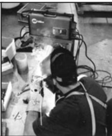
The low amp draw of the Dynasty 200 DX with Auto-Line enabled this fabricator to add eight more TIG machines without any changes to an already stressed primary service.
