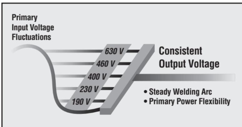
The Auto-Line circuit boosts primary power to a higher, constant voltage. Even if incoming voltage varies widely, the Auto-Line circuit ensures a rock-steady welding or cutting arc.
